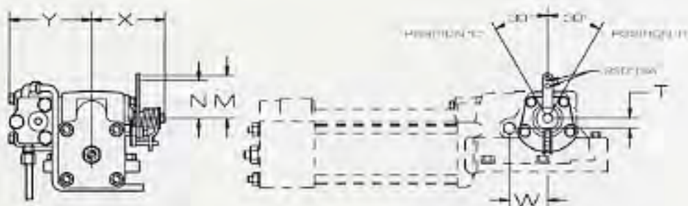
SCISSORS SPRING DETENT
